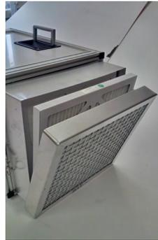
The H13/14 hepafilter can be replaced by following the same procedure as above. If you use the machine daily we would recommend changing the hepafilter once a year. Of course, this depends on the contamination of the air in the environment. At the top of the hepafilter you will find a label with the item number (compare this number with the number on the old filter). Make sure you place the filter as indicated on the label: **↑Airflow**.
