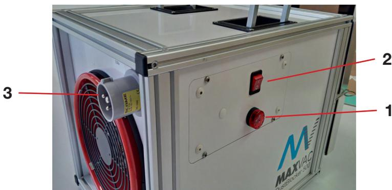
Red led with a warning signal (gives a signal if the H14/G4 filter has to be replaced) (1)
