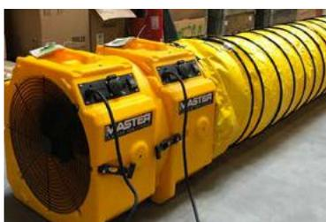
Two connected units increase the air pressure - this allows more than one flex tube to be connected to ventilate over longer distances.
