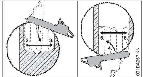
Perform this felling cut when the tree diameter is greater than the cutting length of the chainsaw.
