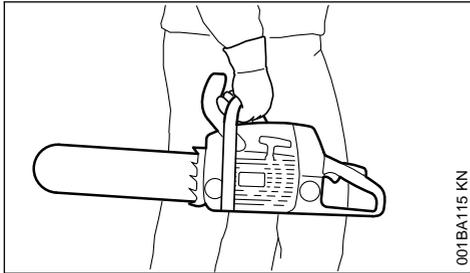
Always carry the chain saw by the handle – with the hot muffler away from your body, the guide bar must point to the rear. To avoid serious burn injuries, avoid touching hot parts of the machine, especially the surface of the muffler.
