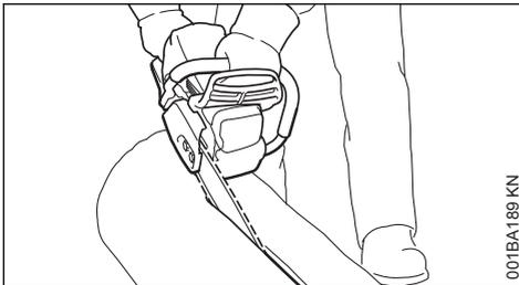
Sawing technique without use of the spiked bumper – risk of pull-in – position the guide bar at as shallow an angle as possible – be especially careful – increased **risk of kickback!**
