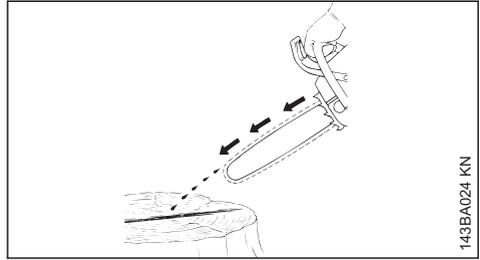
The saw chain must always spin off a small amount of oil.
