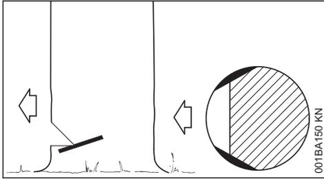
Sapwood cuts in long-fibered softwood help prevent sapwood splintering when the tree falls. Make cuts at both sides of the trunk at same height as bottom of felling notch to a depth of about 1/10 of trunk diameter. On large diameter trees, cut to no more than width of guide bar.
