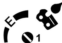
Use the adjusting screw (1) (on underside of machine) to vary the oil feed rate as required.
