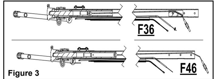
9. Slide pitch cable assembly into top of handle tube (18), guiding cable into top of cable slide (14), F36 handle, see figure #3.
