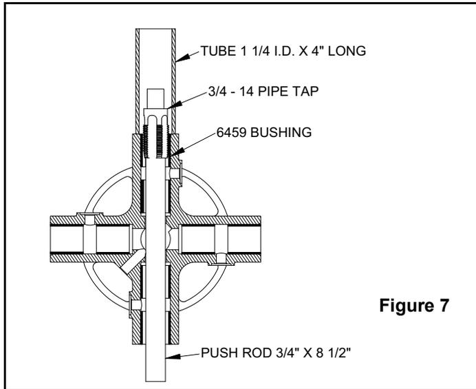
2. Using the opposite end or short end of installation tool #06703, install (4) outer bushings into spider.
