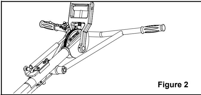
8. Slide activating shaft (11) out of gear assembly (15) and remove handle assembly (9).
