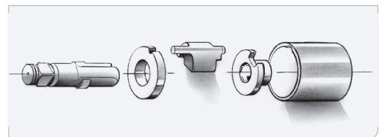
The closed hammer system is constructed, without a loose hammer pin to prevent breakage. The working principle is based on the 1-hammer system which makes 1 impact per rotation at both sides of the anvil.
