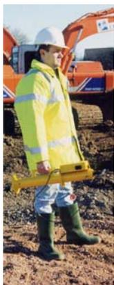
**CBR Measurement:** - Good correlation with results from CBR tests exists. Data from the CIST/884 can be used in a similar manner to results from CBR tests performed in the laboratory and in the field. The CIST/884 display when enabled by the user can directly show the %CBR result based upon Dr Clegg's original pioneering work.
