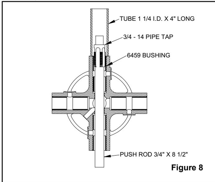
2. Using the opposite end or short end of installation tool #60703, install (4) outer bushings into spider.
