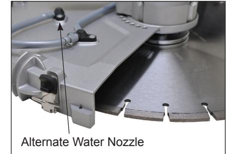
**NOTE:** There is roughly a 1mm or less effective offset (Depending on the width of the diamond segments). Since the blade guard has some degree of flexibility, pushing down slightly brings it all the way to fully flush. In actual cutting, it comes out 100% flush. There has to be a small degree of offset so the blade won't make marks in the base material, in cases where it matters. So to avoid the marks, don't use any downforce. But to get 100% flush, use some downforce.
