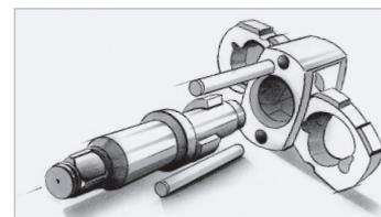
The twin-hammer system makes 2 impacts per rotation at both sides of the anvil. Same principal as the 2-hammer system, manufactured differently.
