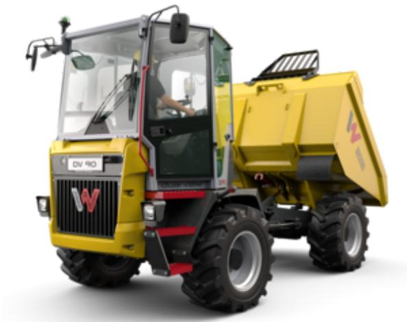
The DV90 Dual View sets new standards in terms of operator and construction site safety, flexibility and economic efficiency. Dual view allows the operator to conveniently and quickly turn the seat with a 180-degree rotation of the entire operator control panel and the seat console. This always gives the operator a perfect view in the direction of travel – during transport, loading and dumping.
