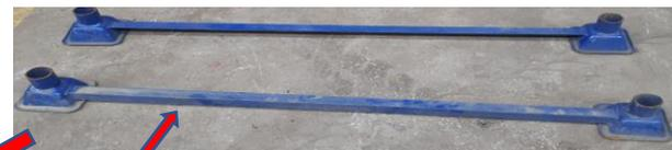
*Foot plate bars can be placed under the stillage by hand making it easy to simply lower the stillage on to with the fork lift truck, 2 x foot plate bars per stillage, if you put the plates under one stillage you can then stack 3 stillage's high when stacking in a warehouse.*
