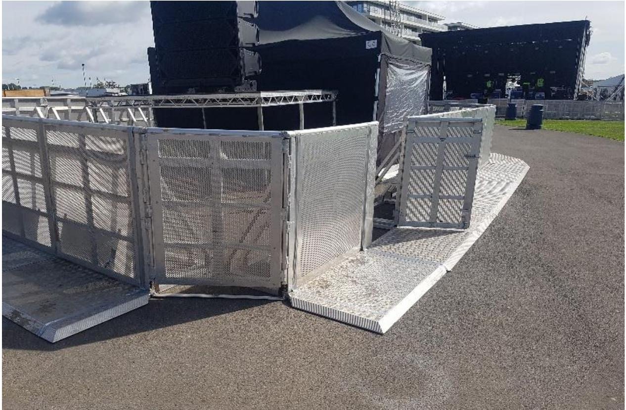
*Image showing a 1m front of stage stage/pedestrian gate being used to create access to the front of house area the front of house area has been barrierd all the way round so the gate is the only access creating a secure area.*
