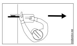
Do not stand in line with the abrasive wheel. Ensure sufficient freedom of movement, especially in construction trenches there must be sufficient space for the user and for the part being cut to fall.
