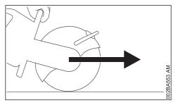
The cut-off machine pulls forward, away from the user, when the abrasive wheel touches the object to be cut from above.
