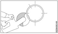
Always start at the bottom, use the upper quarter of the abrasive wheel for cutting
