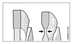
Do not cut into the base course (frequently chipped stones and gravel) when cutting roadway pavement – cutting in chipped stones and gravel is revealed by light-colored dust - excessive undercut may occur as a result - Danger of shatterina!
