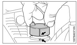
Grip the cap – the cap is closed properly if it cannot be removed and the markings (arrows) on the cap and fuel tank are aligned
