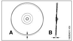
An excessively high radial run-out deviation (A) overloads individual diamond segments, which overheat in the process. This can lead to stress cracks in the parent wheel or to annealing of individual segments.
