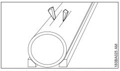
Use wedges and/or leave ridges that are broken after cutting
