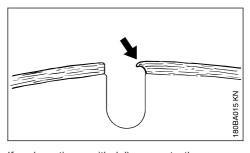
If work continues with dull segments, these may soften due to the high heat generated - the parent wheel is annealed and its strength is compromised - this can lead to stresses that are clearly recognizable by gyrations of the abrasive wheel. Do not continue to use the abrasive wheel - Risk of accident!
