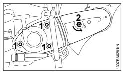
Prior to tensioning of the ribbed V-belt, the nuts (1) must be loosened and the arrow on the tensioning nut (2) must point to  $\bf 0$ .
