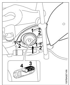
Press the oblong holes (1) in the "cast arm and guard" on to the studs (2), guiding the ribbed V-belt over the front pulley
