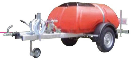
These durable impact resistant polythene tanks are Water Council Approved for drinking water and have internal anti-surge baffles for ease of towing on the highway.
