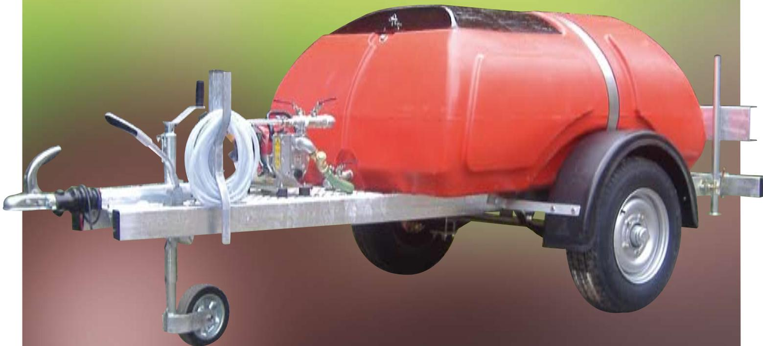
**THIS 1100 LITRE PLASTIC WATER BOWSER COMES COMPLETE WITH A BOOMINATOR SPRAYING SYSTEM, 1" HONDA PETROL PUMP, AND SPRAY GUN. IDEAL FOR WATERING THE GREENS, DAMPING DOWN QUARRIES, RACECOURSES ETC AND IN ANY SITUATION WHERE DUST SUPPRESSION OR WATERING IS REQUIRED.**
