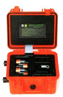
Power Source: Four Alkaline 'D' cells
