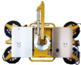
The **Slimliner** is the lightest suction unit with 900 kg capacity. This creates a large overall payload. It combines high capacity with flexibility. Thanks to the 16-cm- flat construction the slimliner allows assembling glass in narrow areas. The suction unit can be extended by 6 to 12 suction plates what doubles capacity from 450 to 900 kg.
