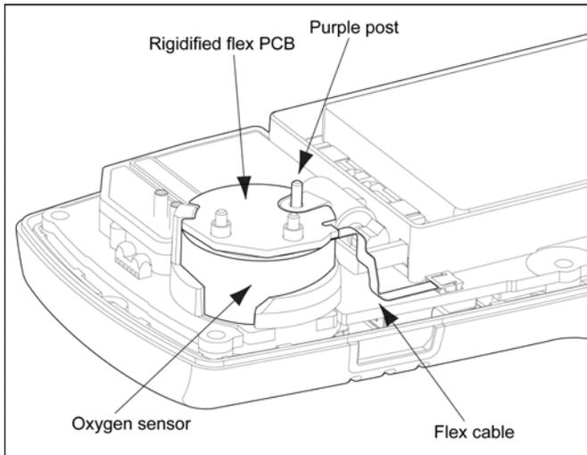
2. Note the placement of the PCB to ensure it is replaced correctly. Remove the two screws on the PCB.
