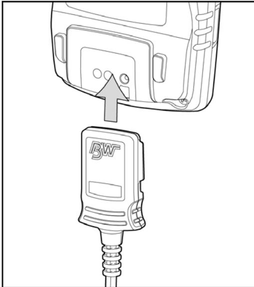
3. Allow the battery to charge for 2-3 hours.
