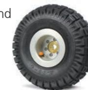
For heavily silted pipes we recommend the optional 250mm Balloon Wheel (QRW250/150), which are also required to centralise the crawler in 1000mm diameter pipes.
