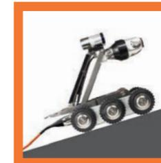
In-built Inclination Sensor
