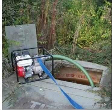
For applications where water contains solids, centrifugal trash pumps are recommended.
