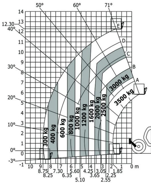
Machine on stabilisers with forks Metric
