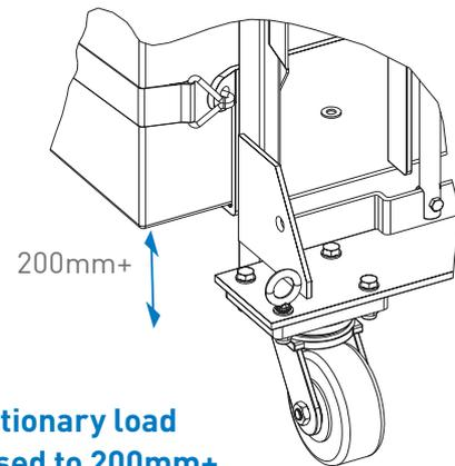
However, if the user wishes to raise the load to a maximum lift height of over 200mm then the straps should be fixed to the Skoots using the eyelets on the toe plate rather than the eyebolts at the rear of the frame before the load is raised. Proceed to raise the load first to the desired height, and then lower it back to the floor when the straps should be reconnected to the eyebolts, crossing the straps over behind the frame before transporting the load.
