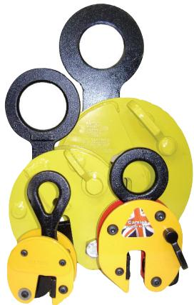
The Camlok brand is over 50 years old and was founded on original, innovative British design and manufacture. It evolved from a general industrial need to lift and transfer steel plate either horizontally, vertically or a combination of both, in a secure and safe manner. This was achieved by using an ingenious 'cam' and jaw mechanism to positively lock the steel plate into a clamping device so it may be suspended from a crane hook.
