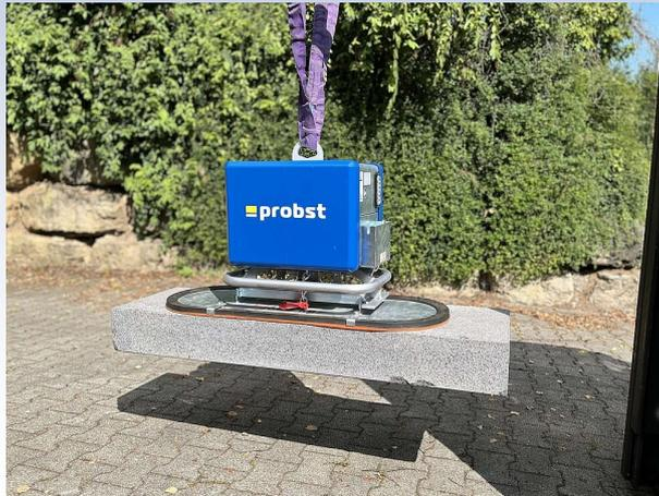
Efficiently installing suction-tight stone slabs, concrete elements, steps and stoneware pipes independently of the power supply.
