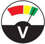
Base units: The volt meter needle should be in the green area. If not, the unit needs to be charged (see page 8)
