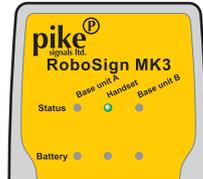
Remote control: The top centre green indicator should be on, the lower centre indicator should be off (see page 7)
