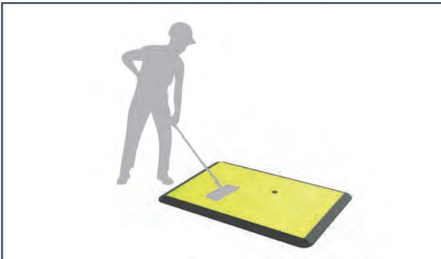
Clean product between every installation to remove debris, and to maintain slip resistance properties.
