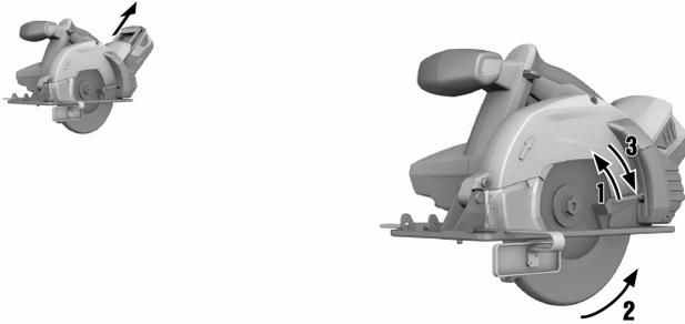
1. Release the cutting depth adjustment clamping lever.
