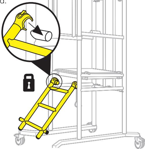
**3** Rotate the ladder down, using the claws as pivots. Locate the bottom of the ladder over the base frame as shown below.
