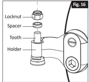
**7.3.2 Replacing Teeth****Inspection Check:**
