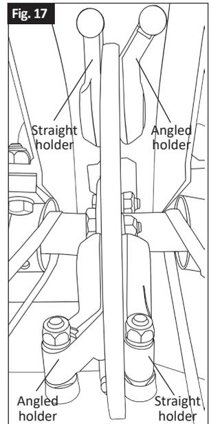
The holders must be fitted alternately, eg, the first pair would be a straight holder and an angled holder, then the second pair would be an angled holder and a straight holder, and so on.
