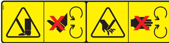
**Danger! Moving blades. Do not remove safety guards whilst engine is running. Keep hands and feet away.**
