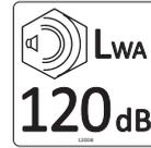
Maximum sound power level (LWA). Ear protection must be worn when the machine is in use.
